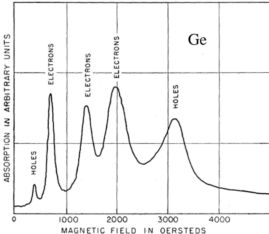
Cyclotron frequency  $\omega_c = \frac{qB}{m}$
