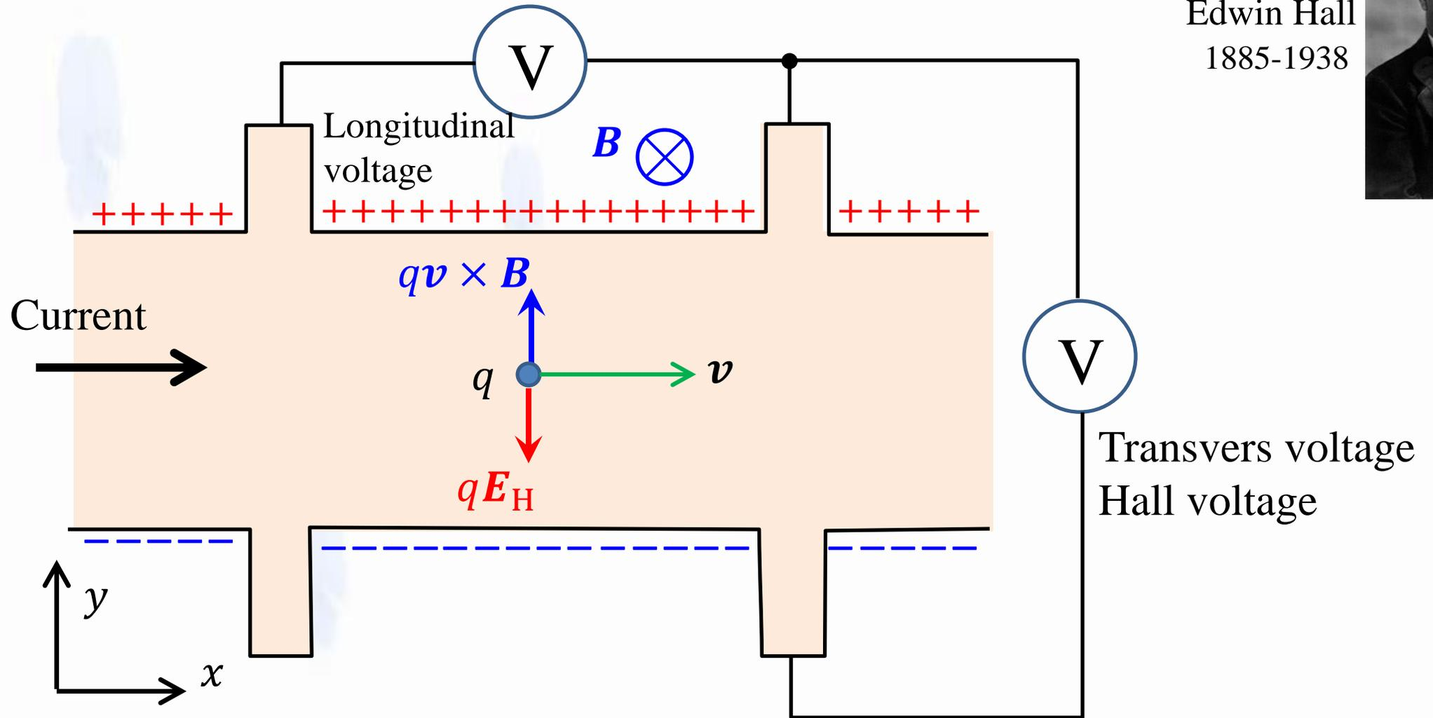
$$R_{xx} = \frac{\text{(longitudinal voltage)}}{\text{(current)}} \quad \text{(longitudinal resistance)}$$
