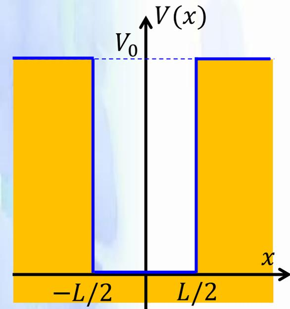
Outside the well:  $\left[ -\frac{\hbar^2}{2m} \frac{d^2}{dx^2} + V_0 \right] \psi = E\psi, \quad x \leq -\frac{L}{2}, \frac{L}{2} \leq x, \quad \kappa \equiv \frac{\sqrt{2m|E - V_0|}}{\hbar}$
