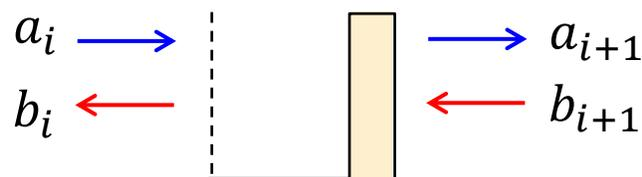
$$M_d(k) = \begin{pmatrix} e^{ikW} & 0 \\ 0 & e^{-ikW} \end{pmatrix} \begin{pmatrix} m_{11} & m_{12} \\ m_{21} & m_{22} \end{pmatrix} = \begin{pmatrix} m_{11}e^{ikW} & m_{12}e^{ikW} \\ m_{21}e^{-ikW} & m_{22}e^{-ikW} \end{pmatrix}$$
