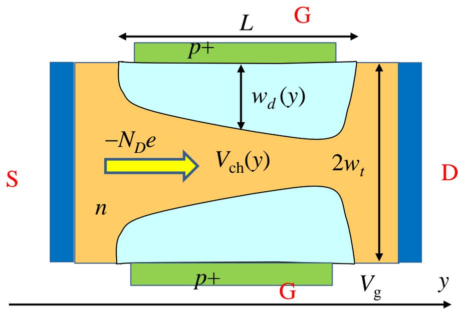
$$V(y) = V_g + V_{bi} - V_{ch}(y)$$
