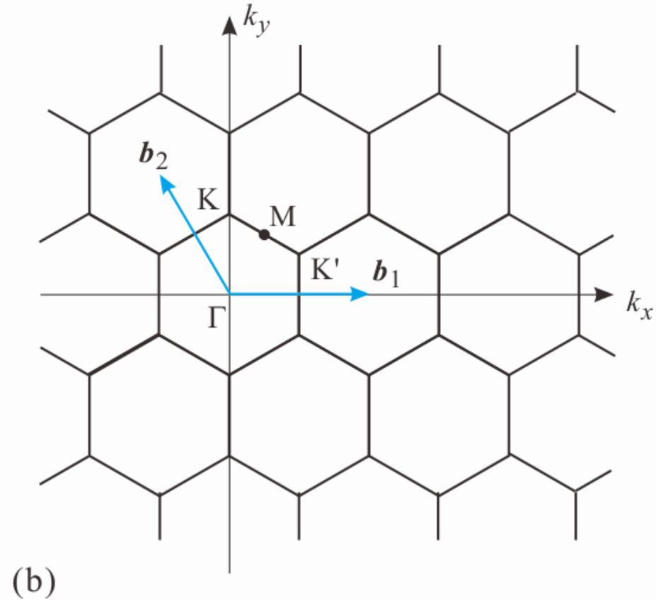
$$\mathbf{b}_1 = \begin{pmatrix} 4\pi/\sqrt{3}a \\ 0 \end{pmatrix}, \quad \mathbf{b}_2 = \begin{pmatrix} -2\pi/\sqrt{3}a \\ 2\pi/a \end{pmatrix}$$
