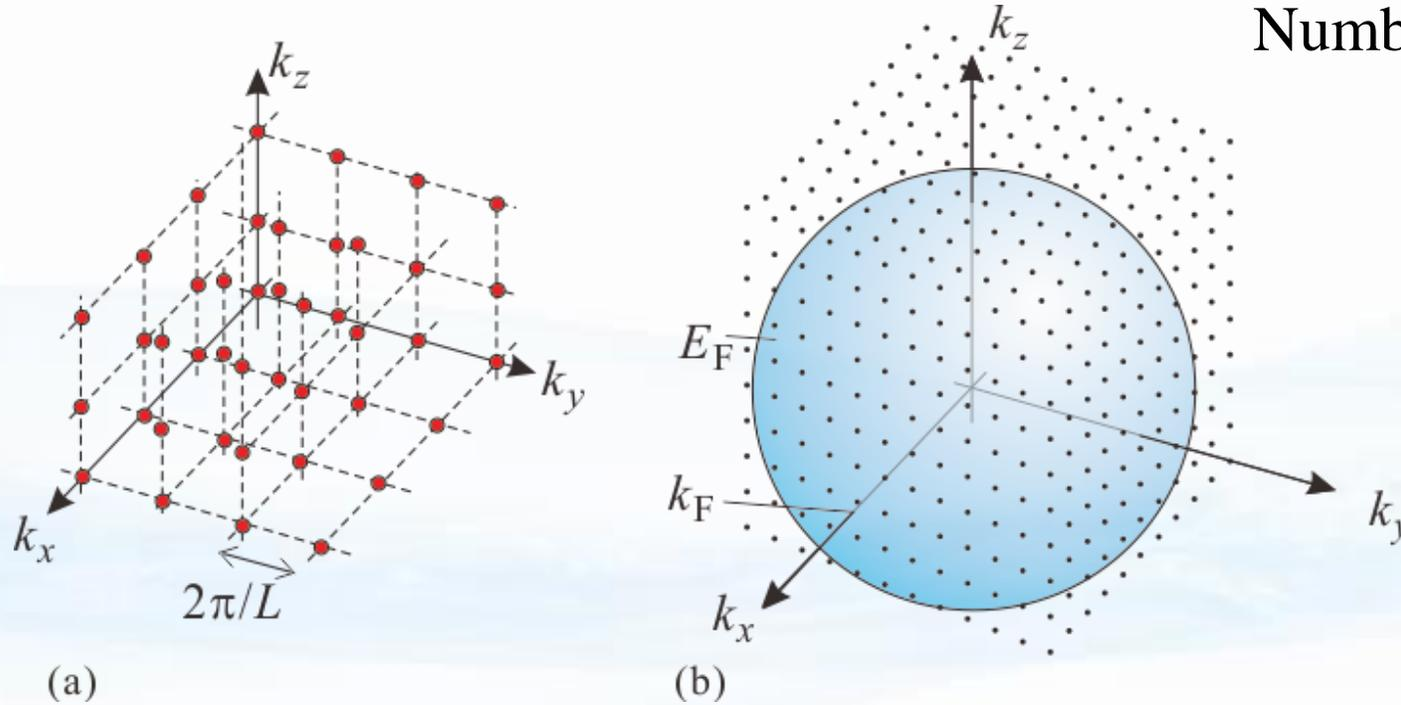
$$\begin{aligned} \mathcal{D}(E) &= \frac{1}{L^d} \left( \frac{L}{2\pi} \right)^d \frac{dV_d(k)}{dE} \\ &= \frac{1}{(2\pi)^d} \frac{dV_d(k)}{dk} \frac{dk}{dE} \\ &= \frac{1}{(2\pi)^d} \frac{m_0}{\hbar^2} \frac{dV_d(k)}{kdk} \end{aligned}$$
