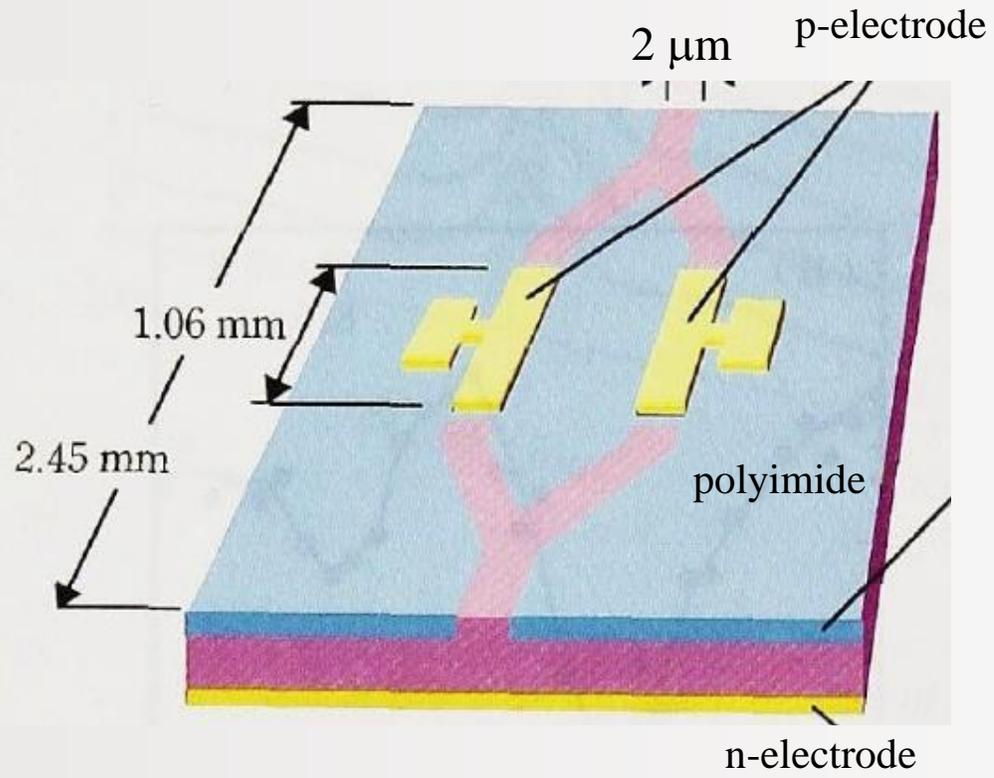
Voltage control of optical output through interference
