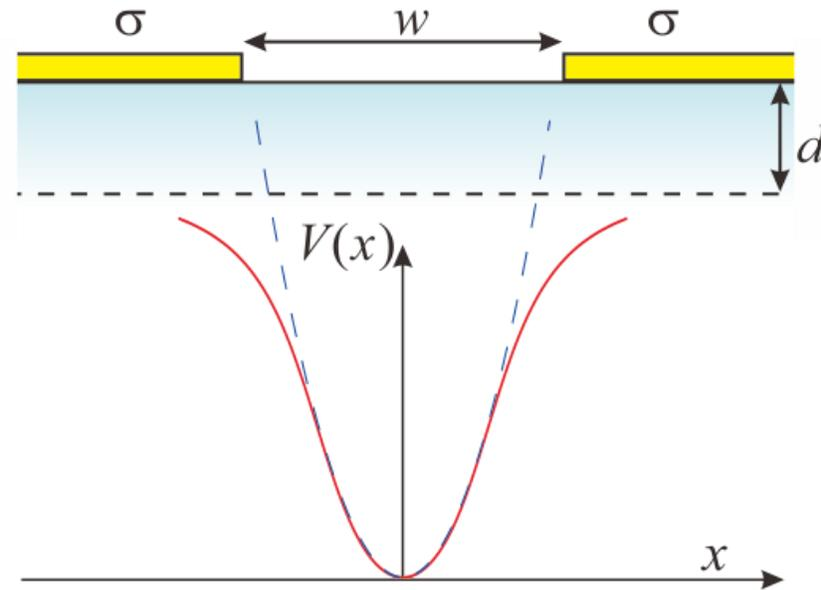
Two-dimensional electrons are pinched with depletion layers from Schottky gates to a one-dimensional system.
