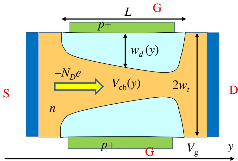
$$V(y) = V_g + V_{bi} - V_{ch}(y)$$
