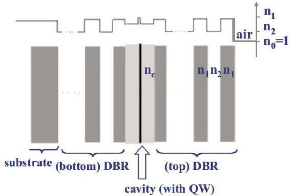
$$T = \frac{(1 - R_1)(1 - R_2)}{[1 - \sqrt{R_1 R_2}]^2 + 4\sqrt{R_1 R_2} \sin^2(\phi/2)}$$
