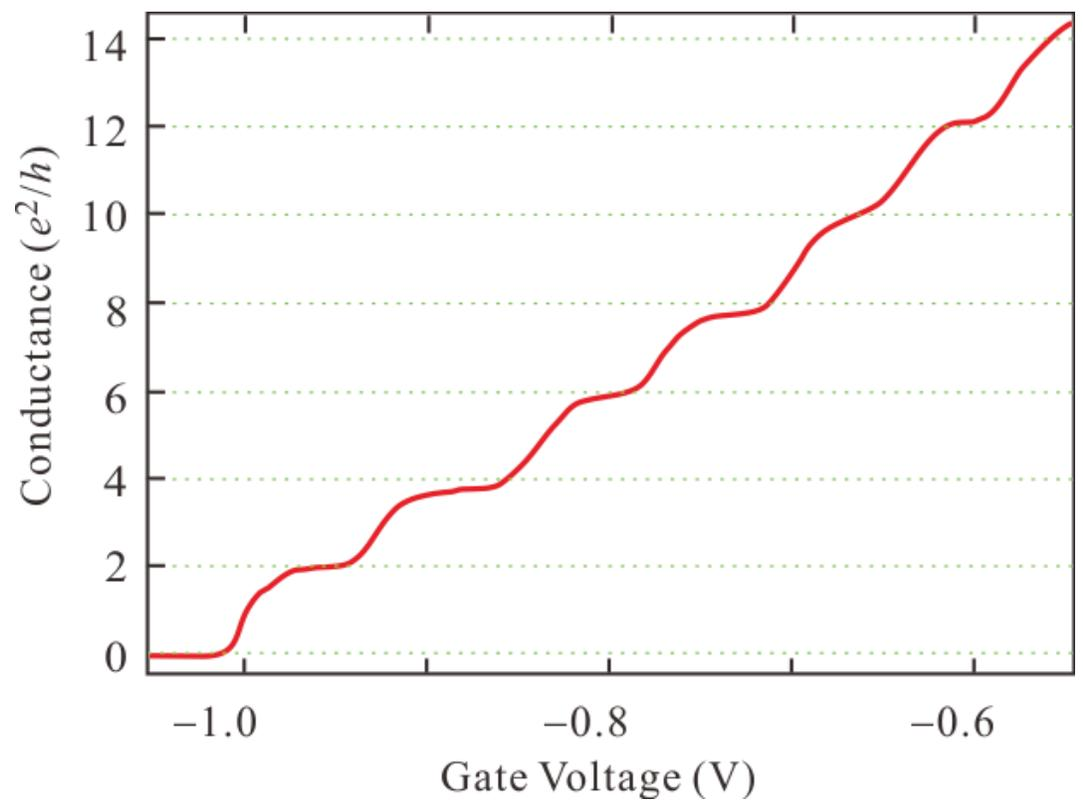
Transmissible one-dimensional system: **Conductance Channel**
