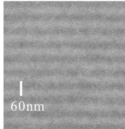
STEM image of AlAs (30 nm)/GaAs (30nm) superlattice
