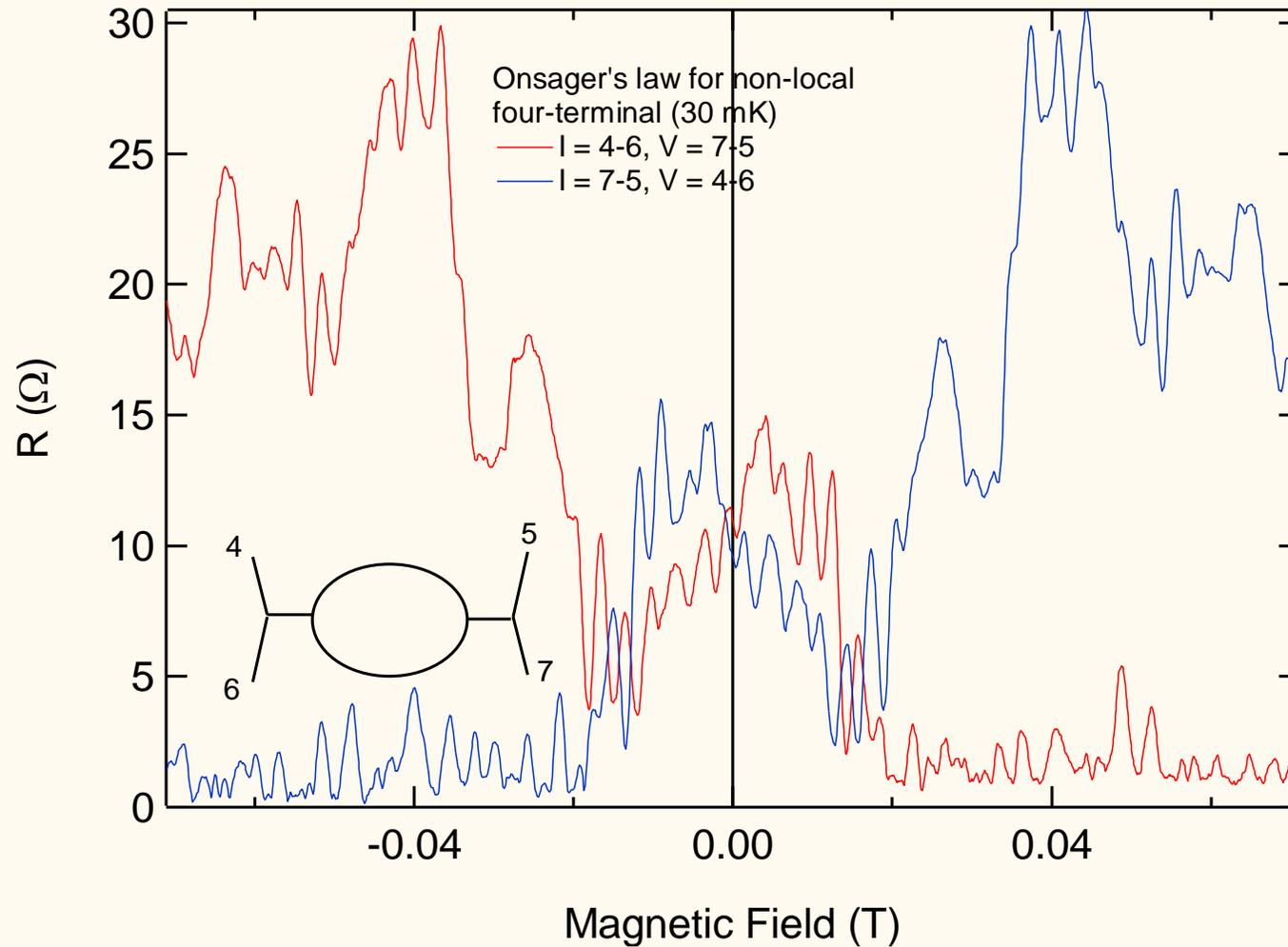
Magnetoresistance: Universal conductance fluctuation including AB oscillation
