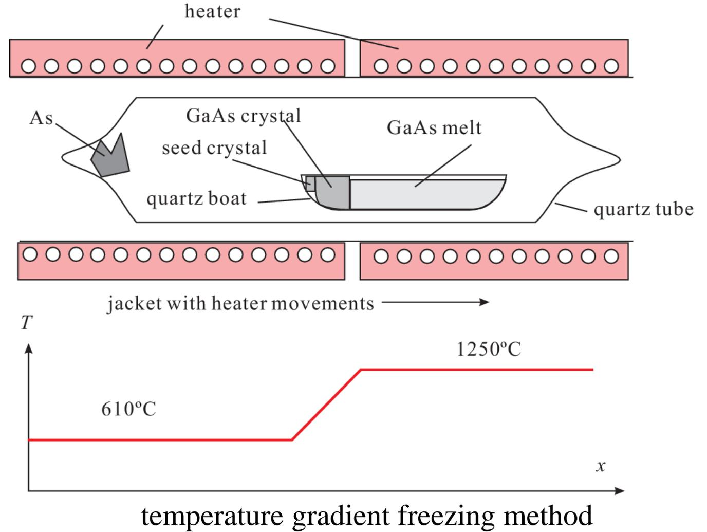
temperature gradient freezing method
