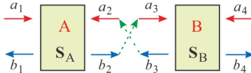
$$\begin{pmatrix} b_1 \\ b_2 \end{pmatrix} = S_A \begin{pmatrix} a_1 \\ a_2 \end{pmatrix} = \begin{pmatrix} r_L^{(A)} & t_R^{(A)} \\ t_L^{(A)} & r_R^{(A)} \end{pmatrix} \begin{pmatrix} a_1 \\ a_2 \end{pmatrix},$$
