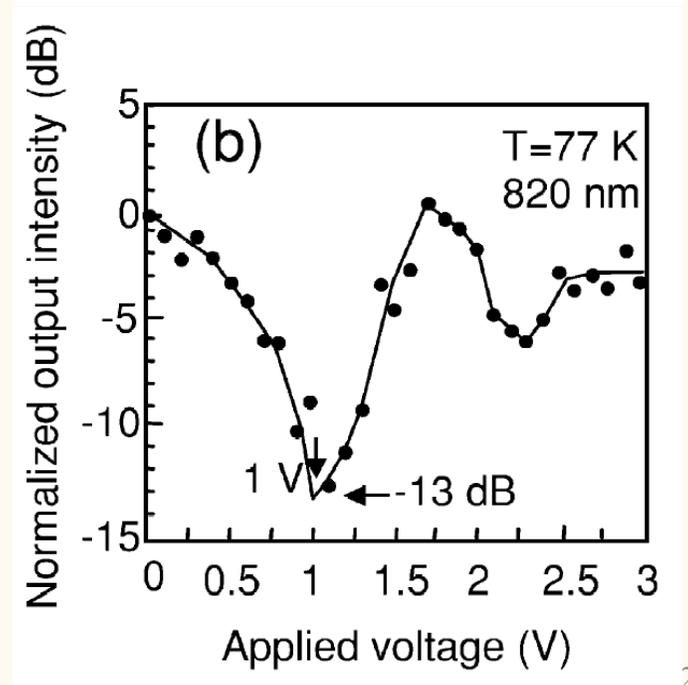
Katsuyama, Hosomi, Micro. Eng. **63**, 23 (2002). Voltage control of optical output through interference
