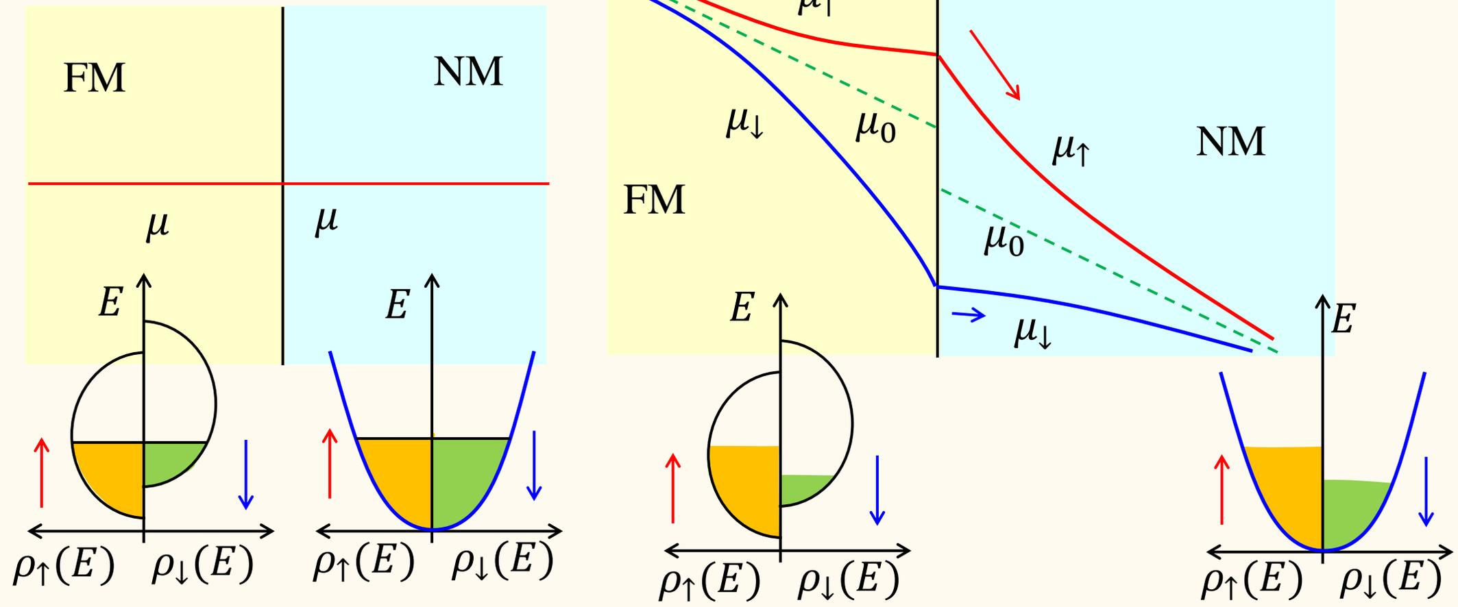
$$\mu_s^M = a^M + b^M x \pm \frac{c^M}{\sigma_s^M} \exp\left(\frac{x}{\lambda_{sf}^M}\right) \pm \frac{d^M}{\sigma_s^M} \exp\left(-\frac{x}{\lambda_{sf}^M}\right) \quad M = F, N$$
