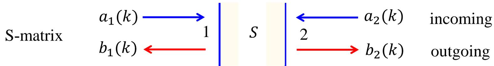
$$\begin{pmatrix} b_1(k) \\ b_2(k) \end{pmatrix} = S \begin{pmatrix} a_1(k) \\ a_2(k) \end{pmatrix} = \begin{pmatrix} r_L & t_R \\ t_L & r_R \end{pmatrix} \begin{pmatrix} a_1(k) \\ a_2(k) \end{pmatrix}$$
