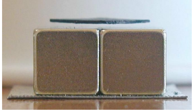
Magnetic levitation of graphite
